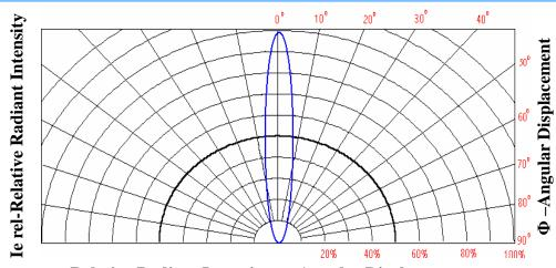
Relative Radiant Intensity vs .Angular Displacement
