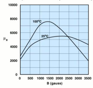
Measured on an 18/10/6mm toroid at 10kHz.
