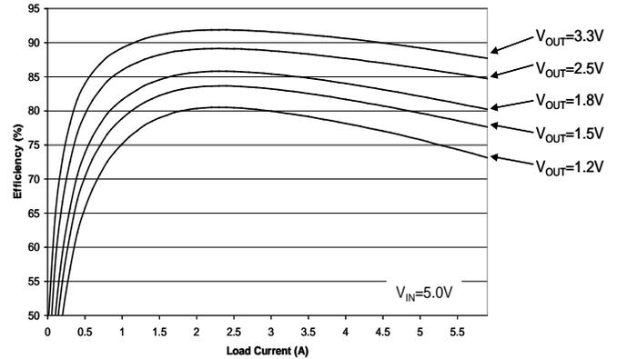
Efficiency vs. Load,  $V_{IN} = 5.0V$ .; Load = 0-6A.
