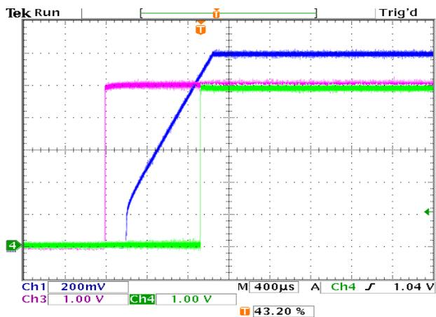
Start up waveforms  $V_{IN}=5.0V$ ,  $V_{OUT}=1.2V$ ,  $C_{SS}=15nF$ ,
