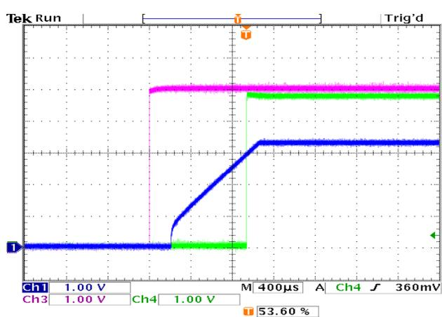
Start up waveforms  $V_{IN}=5.0V$ ,  $V_{OUT}=3.3V$ ,  $C_{SS}=15nF$ ,
