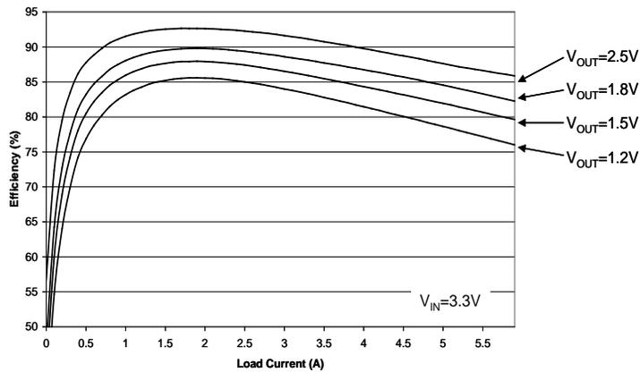
Efficiency vs. Load,  $V_{IN} = 3.3V$ .; Load = 0-6A.
