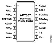
Figure 2. Pin Configuration
