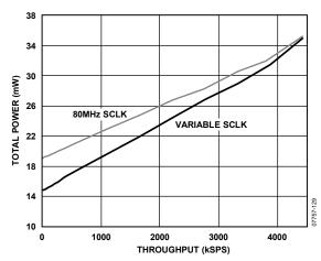
Figure 29. Power vs. Throughput Rate
