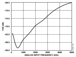
Figure 18. THD vs. Analog Input Frequency
