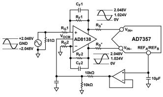
\*MOUNT AS CLOSE TO THE AD7357 AS POSSIBLE AND ENSURE THAT HIGH PRECISION  $R_S$  RESISTORS ARE USED.  $R_S-33\Omega$ ;  $R_G1=R_{F1}=R_{F2}=499\Omega$ ;  $C_F1=C_{F2}=39pF$ ;  $R_G^2=523\Omega$
