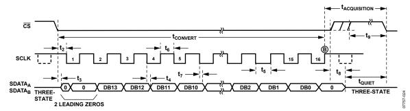
Figure 30. Serial Interface Timing Diagram
