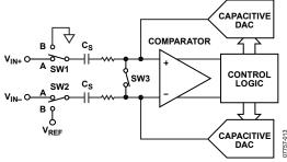
Figure 14. ADC Acquisition Phase
