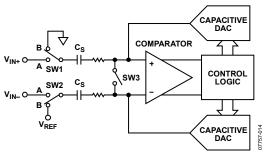
Figure 15. ADC Conversion Phase
