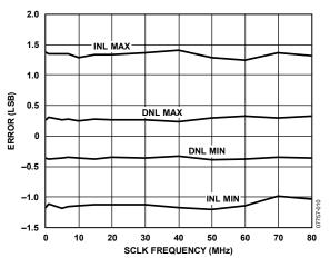
Figure 10. Linearity Error vs. SCLK Frequency
