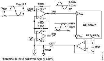
Figure 21. Dual Op Amp Circuit to Convert a Single-Ended Unipolar Signal into a Differential Signal
