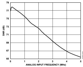
Figure 7. SNR vs. Analog Input Frequency
