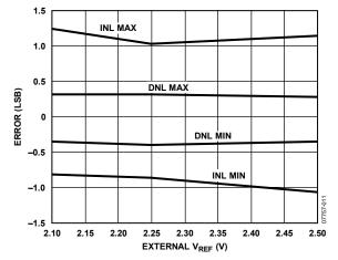
Figure 11. Linearity Error vs. External  $V_{\text{REF}}$
