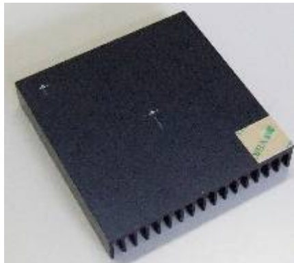
Affixing a double-coated adhesive tape to a heat sink fin Bonding and fixing a power LED onto the tape
