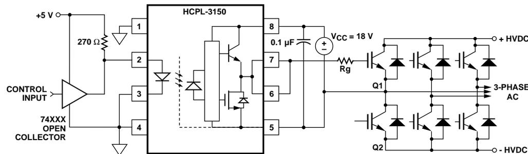
Figure 25a. Recommended LED Drive and Application Circuit.
