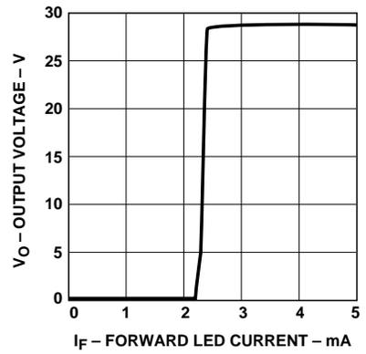
Figure 15. Transfer Characteristics.
