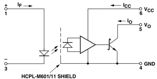
USE OF A 0.1  $\mu$ F BYPASS CAPACITOR MUST BE CONNECTED BETWEEN PINS 6 AND 4 (SEE NOTE 1).
