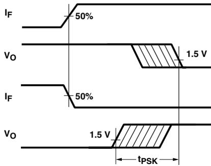
Figure 15. Illustration of Propagation Delay Skew -  $t_{PSK}$ .
