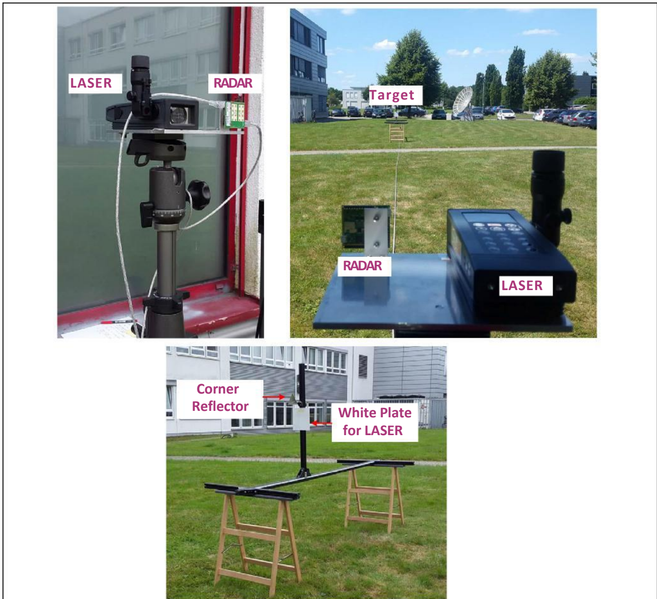
Figure 32 Distance2Go – Outdoor Measurement Setup
