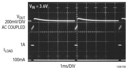
図8. GSM負荷過渡応答。低掃引速度(1ms/DIV)
