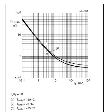
Fig.7 Collector-emitter equivalent on-resistance
