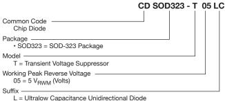
LC = Ultralow Capacitance Bidirectional Diode
