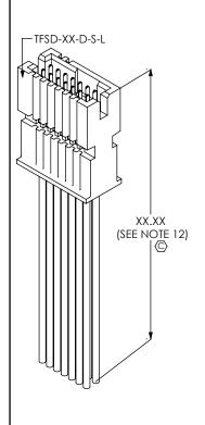
FIG 5 -DL: DOUBLE END WITH FRICTION LOCK (TFSDX-07-28-XX-XX.XX-DL-NUS SHOWN) (DIFFERENT AS SHOWN, OTHERWISE SAME AS FIG 1)
