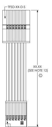
FIG 4 -SL: SINGLE END WITH FRICTION LOCK (TFSDX-07-28-XX-XX.XX-SL SHOWN) (DIFFERENT AS SHOWN, OTHERWISE SAME AS FIG 1)
