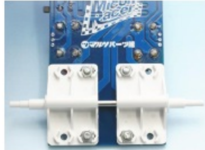
Completion of mounting axle and axle holders on Micon Racer2 board
