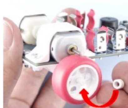
Mount tires to Micon Racer2 with tire fixing parts.
