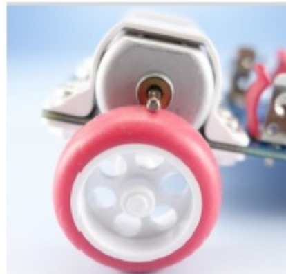
While it's placed on, motor shaft touches tire, and power is translated.
