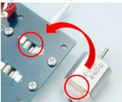
Place motor as putting boss of motor into cutout
