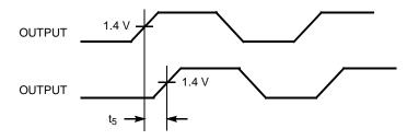
Figure 7. Input-Output Propagation Delay
