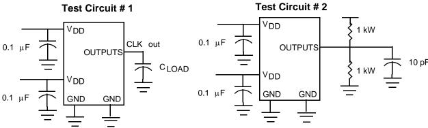
For parameter t8 (output slew rate) on -1H devices
