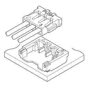
This ACH connector is compact and low profile type, height: 1.4mm and width 4.3mm,1.2mm pitch wire-to-board connector.
