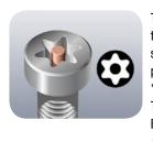
TORX<sup>®</sup> tools with a borehole prevent the unauthorised unfastening of safety screws. The screws contain a pin that protrudes into the drive profile so that "normal" TORX<sup>®</sup> tools cannot be used. This pin fits into the borehole of TORX<sup>®</sup> B0 tools allowing safety screws to be unfastened.
