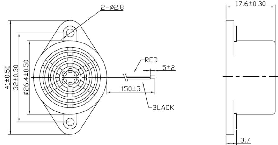
Dimensions Unit: mm Tolerance: ±0.5mm
