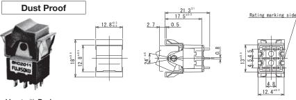
Mount with Rocker Terminal numbers are not shown on the bottom of the switch.
