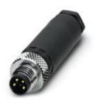
Connector, Universal, 4-position, Plug straight M8, A-coded, Screw connection, knurl material: Nickel-plated brass, external cable diameter  $3.5~\mathrm{mm}$  ...  $5~\mathrm{mm}$
