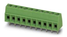
Printed circuit terminal block, nominal current: 10 A, rated voltage: 160 V, pitch: 3.5 mm, no. of positions: 6, mounting: Soldering, type of connection: Screw connection, connection direction from the conductor to the PCB:  $0^{\circ}$
