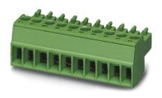
Plug component, nominal current: 8 A, rated voltage: 160 V, pitch: 3.5 mm, no. of positions: 10, type of connection: Screw connection
