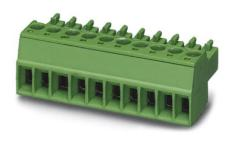
Plug component, nominal current: 8 A, rated voltage: 160 V, pitch: 3.5 mm, no. of positions: 12, type of connection: Screw connection
