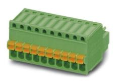
Plug, nominal current: 4 A, rated voltage: 100 V, pitch: 2.5 mm, number of positions: 7, connection method: Spring-cage connection
