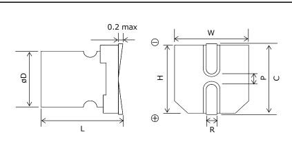
Unit : mm Size L +0.1 -0.4 P±0.2 øD±0.5 W±0.2 H±0.2 C±0.2 R code В6 5.0 5.9 5.3 5.3 6.0 0.6 to 0.8 1.4 7.3 0.6 to 0.8 C6 6.3 5.9 6.6 6.6 2.1 8.0 6.9 8.3 8.3 9.0 0.6 to 0.8 3.2 **E7** 8.0 10.0\*1 8.3 8.3 9.0 0.8 to 1.1 E10 3.2 0.8 to 1.1 E12 8.0 11.9 8.3 8.3 9.0 3.2 F10 10.0 10.0\*1 10.3 10.3 11.0 0.8 to 1.1 4.6 F12 10.0 10.3 0.8 to 1.1 4.6 12.6 10.3 11.0 \*1:±0.5
