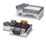
D-SUB connector, 9-pos., male connector, cable entry < 35°, bus system: PROFIBUS DP up to 12 Mbps, termination resistor can be switched on via slide switch, pin assignment: 3, 5, 6, 8; screw connection terminal blocks
