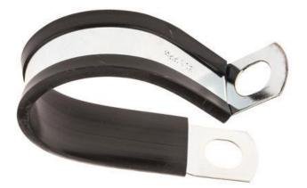
MATERIAL: MILD STEEL TO BS EN 1030 FEPO FINISH: BRIGHT ZINC PLATE TO BS1706 Fe/ZN5c 1A LINER: PVC BLACK TO BS2571 TEMPERATURE RANGE -25°C TO +105°C
