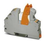
Pre-assembled relay module with push-in connection, consisting of: relay base, power contact relay, plug-in display/suppressor module, and retaining bracket. Contact type: 2 PDTs. Input voltage: 230 V AC
