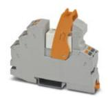
Pre-assembled relay module with push-in connection, consisting of: relay base, power contact relay, plug-in display/suppressor module, and retaining bracket. Contact type: 1 PDT. Input voltage: 230 V AC
