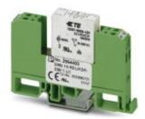
Relay module, with soldered-in miniature switching relay, contacts (AgNi): Medium to large loads, 1 N/O contact, input voltage 230 V AC/DC
