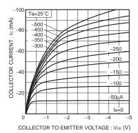
Fig.3 Grounded emitter output characteristics (II)
