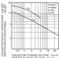
$\begin{array}{c} \text{COLLECTOR TO BASE VOLTAGE: VCB (V)} \\ \text{EMITTER TO BASE VOLTAGE: VEB (V)} \\ \text{Fig.9 Collector output capacitance vs.} \end{array}$
