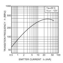
Fig.8 Gain bandwidth product vs. emitter current
