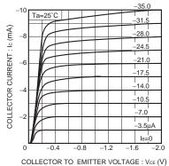
Fig.2 Grounded emitter output
