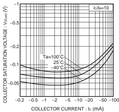
Fig.7 Collector-emitter saturation voltage vs. collector current (II)
