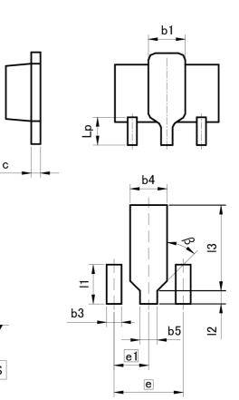
Pattern of terminal position areas [Not a recommended pattern of soldering pads]
