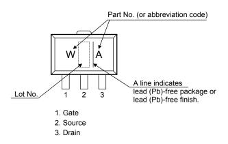
This device is sensitive to electrostatic discharge.
