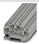
Double-level spring-cage terminal block, Cross section: 0.08 mm² - 1.5 mm², AWG: 28 - 16, Connection type: Spring-cage connection, Width: 4.2 mm, Color: gray, Mounting type: NS 35/7,5, NS 35/15
