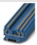
Feed-through terminal block, nom. voltage: 800 V, nominal current: 24 A, connection method: Push-in connection, number of connections: 3, cross section: 0.14 mm² - 4 mm², AWG: 26 - 12, width: 5.2 mm, height: 35.2 mm, color: blue, mounting type: NS 35/7,5, NS 35/15
