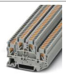
Double-level terminal block, connection method: Push-in connection, cross section: 0.14 mm² - 4 mm², AWG: 26 - 12, width: 5.2 mm, color: gray, mounting type: NS 35/7,5, NS 35/15
