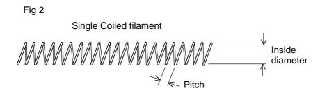
The closer the spacing of the coils, (known as the pitch), then the hotter the filament can operate.
