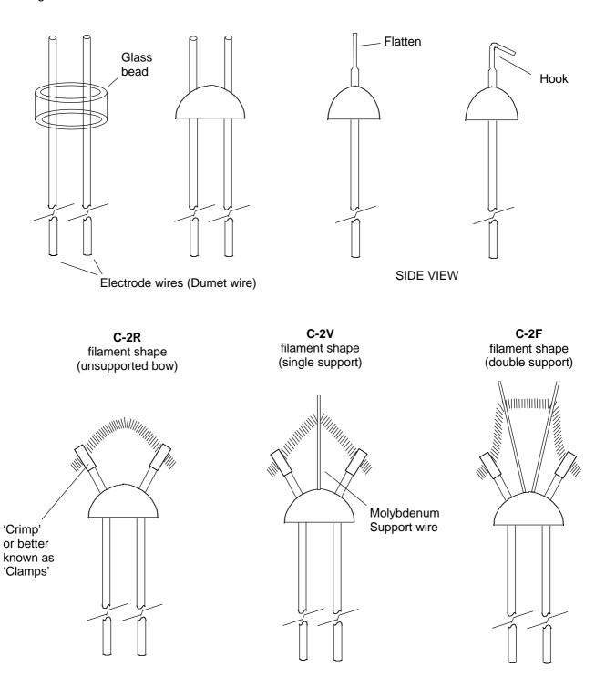
• The filament when mounted to the electrodes is known as the 'Mount'.
