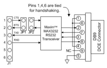
Figure 1. PmodRS232 block diagram.
