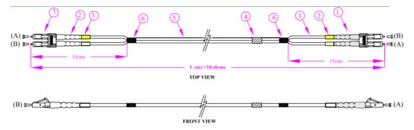
**Optical Performance** (IEC 61300-3-4): **Multimode** (@ 1300nm) LC : Max. IL - 0.30dB Typical: 0.20dB **Singlemode:** (@1310nm and/or 1550nm) LC : Max. IL - 0.30dB Typical: 0.20dB Return Loss: >50dB
