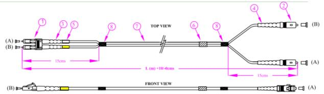
Connector: SC Clips shall be mounted to the connector to make it duplex.
