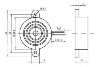
Dimensions Unit: mm Tolerance: ±0.5mm
