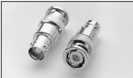
Model 6172: 2-slot male to 3-lug female triax adapter. For use in adapting Models 7065 and 250INT inputs to 3-slot triax plugs.
