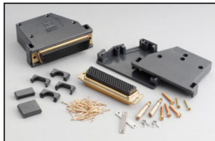
Model 3792-KIT104-R: 104-pin male D-sub connector kit that contains two male D-sub connectors with housings and 208 solder-cup contacts. Use for assembly of custom cable and harnesses compatible with Series 3700A plug-in cards.
