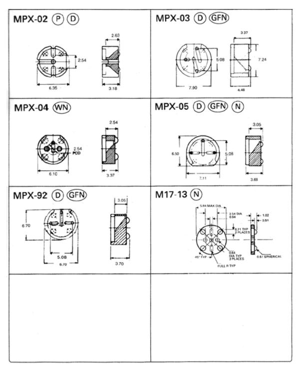
Key D = Glass Filled Polyester GFN = Glass Filled Nylon P = Polypropylene
