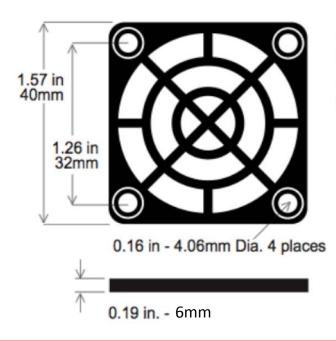
Material: Plastic - reinforced ABS UL approved Rating UL94V-O
