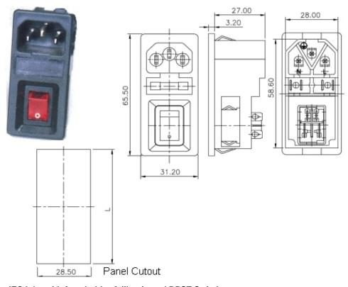
IEC Inlet with fuse holder & illuminated DPST Switch
