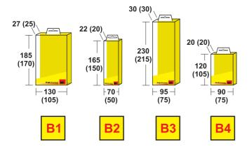
The figures given in the drawings for width, height and depth are approximate **outer (inner)** dimensions in millimetres. In the catalogue, the employed blister size is indicated by the symbol **B1** to **B4** beside each article.
