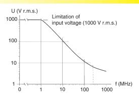
The rated voltage of the 10:1 probe dividers is frequency-dependent.
