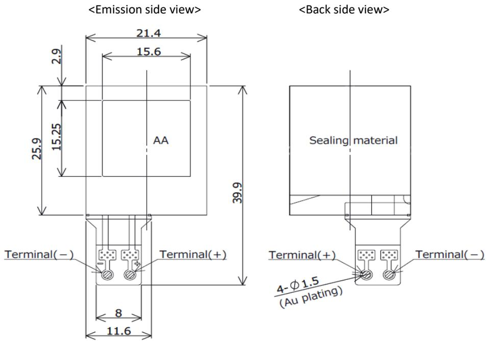
Tolerances of dimensions are  $\pm 0.3\text{mm}$
