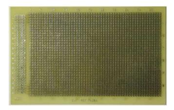
Double sided Epoxy FR4 thickness 15/10th. Fully pated single sided tinned square pads 2 mm $^2$ , drilled Ø 1 mm with connector DIN 41612. The other side fully copper clad for shielding. Milling of the holes to avoid circuit-breaker. Size: 100 x 160 mm.
