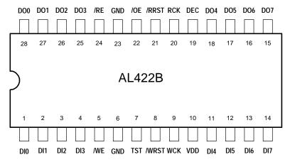
AL422-04 422B pinout diagram
