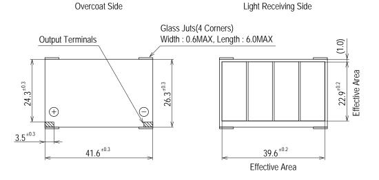
Note: Glass Substrate Thickness : 1.1mm Module Thickness : 1.3mm max Accepts normal soldering for bending.
